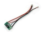
**Code G5K000P5**: Micro-B USB mounted on white round support 12mm in diameter and 7mm high with 10cm AWG22 cable and connector.
