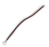
**Code G5K000X7L** with 6mm external diameter and 3mm inner diameter and 16cm of cable and micro-connector. Short touch function ON and OFF. Long touch for regulation. It does not save memory. It must always be connected before battery.
