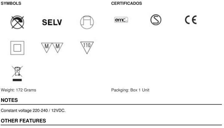
Length (mm): 165 High (mm): 30 Voltage In (Vac): 220~240 Intensidad Out (A): 0~2.5 Power (W): 0~30 Ingress Protection: IP20 Power factor: 0.95
