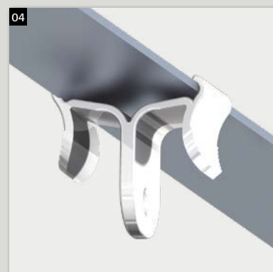
04 T track-clip with bore Off-white similar to RAL 9001 bore 4 mm WLL (DIN 18168) 5 kg Art. no. 029.005.579
