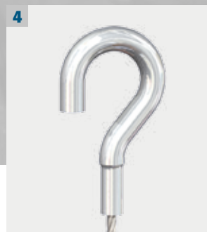
4 Wire hook Opening gap 4 mm WLL 10 kg
